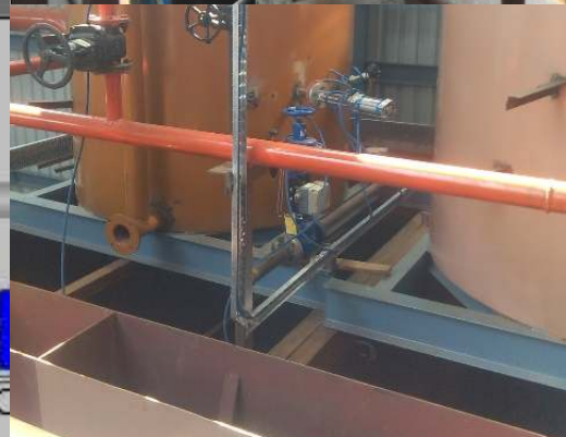
Auto Retracting Self Cleaning Brix Sensor installed on Batch Type Vacuum Pan
