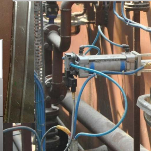
Auto Retracting Self Cleaning Brix Sensor installed on Continuous Vacuum Pan & Sugar Melter in Picture below
